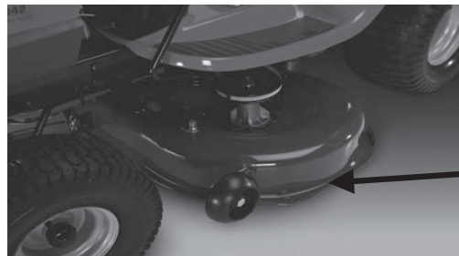
Stamped Deck Shell below, NOT reinforced
