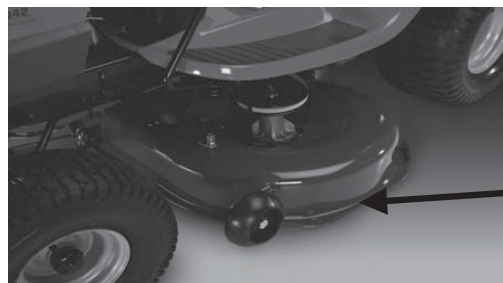
Stamped Deck Shell below, NOT reinforced
