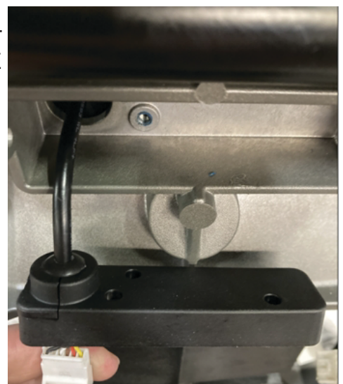
GROMMET PLACEMENT IN SUBFRAME
