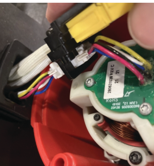
PHASE WIRES AND HALL WIRES CONNECTED
