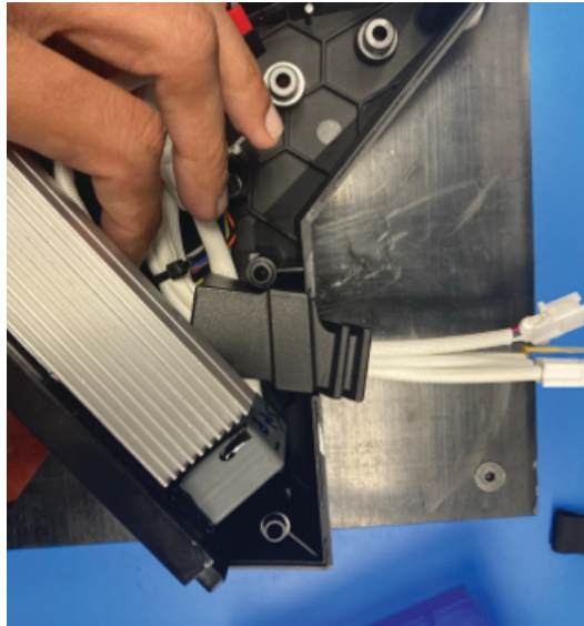
PHASE WIRES AND BATTERY PLUS/MINUS ROUTING
