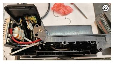
23. Add dielectric grease to cover pins in remaining female connector on PCB.
