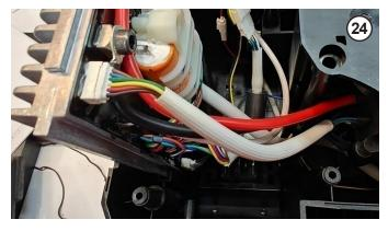
24. Fully seat wire bundle connector from battery rail.
