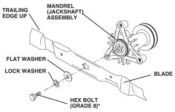
\*A GRADE 8 HEAT TREATED BOLT CAN BE IDENTIFIED BY SIX LINES ON THE BOLT HEAD. FIG. 1
