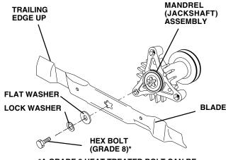
\*A GRADE 8 HEAT TREATED BOLT CAN BE IDENTIFIED BY SIX LINES ON THE BOLT HEAD.
