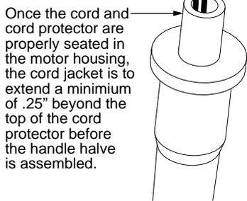
Once the cord and cord protector are properly seated in the motor housing, the cord jacket is to extend a minimum of .25" beyond the top of the cord protector before the handle half is assembled.
