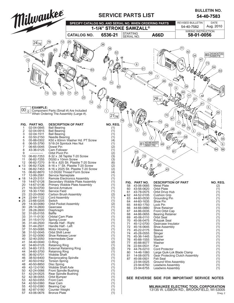
NOTES: FIG. Bearing to be installed with seal towards commutator. 4,31 Press needle bearing flush ±.005 with inner surface of diaphragm.
