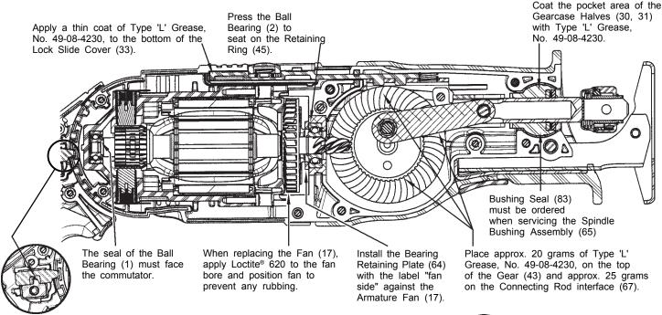
Coat the pocket of the Lock Slide (74) with Type 'L' Grease, No. 49-08-4230.
