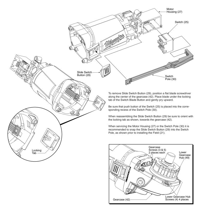
When servicing the Gearcase (42), first remove the four Screws (4) and Lower Gearcase Hub (49) to prevent damage to the bottom two Screws (5) that secure the Gearcase.
