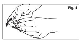
To remove collet from nut, hold nut firmly with one hand and press the collet to one side with the other hand (Fig. 4).
