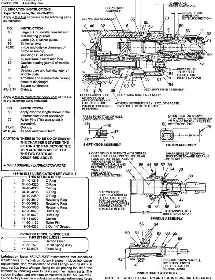
NOTE: THE WOBBLE SHAFT #59 AND THE INTERMEDIATE GEAR #42 ARE TO BE PRESSED FLUSH TO EACH OTHER, SO THAT THE WOBBLE SHAFT IS STILL ABLE TO REVOLVE FREELY - WITH .005" MAXIMUM AXIAL PLAY ON THE INTERMEDIATE SHAFT #43.
