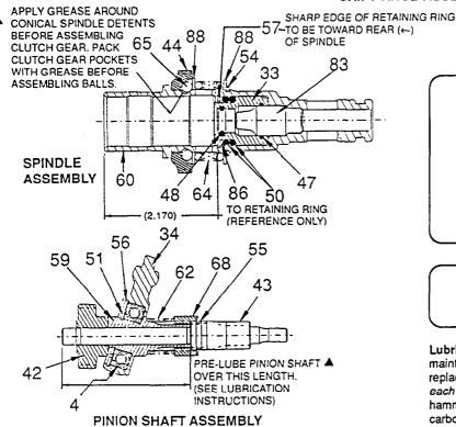
NOTE: THE WOBBLE SHAFT #59 AND THE INTERMEDIATE GEAR #42 ARE TO BE PRESSED FLUSH TO EACH OTHER, SO THAT THE WOBBLE SHAFT IS STILL ABLE TO REVOLVE FREELY - WITH .005" MAXIMUM AXIAL PLAY ON THE INTERMEDIATE SHAFT #58
