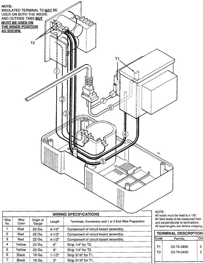
All leads must be held to  $\pm 1/8$ ". All field leads to be measured from and perpendicular to laminations.
