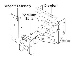
When removing the support assembly—pull outward on the stop bracket to release it from and the drawbar and slide support assembly up.
