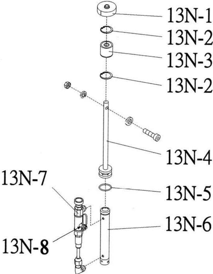
10.2.2 HVBS-7MW Cylinder Assembly – Parts List
