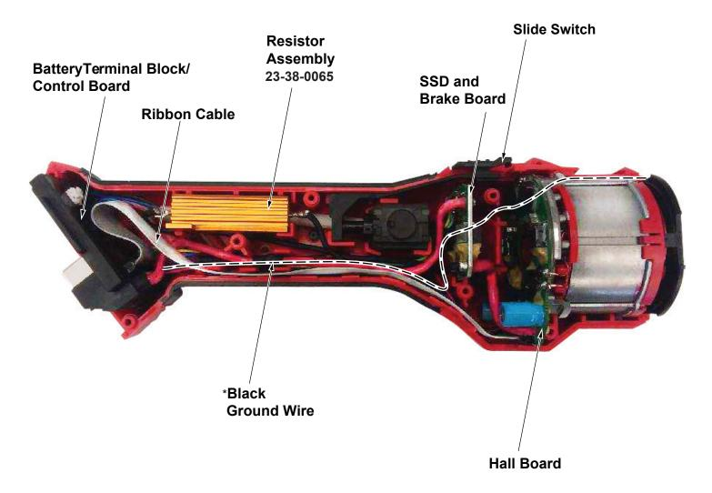
\*The Black Ground Wire demonstrated in above diagram is placed toward bottom and in the back of all other wires and components assembled in the main housing.
