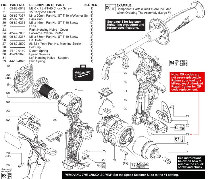
REMOVING THE CHUCK SCREW: Set the Speed Selector Slide to the #1 setting.
