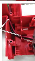
Place the red and black fan wires into wire traps as shown.
