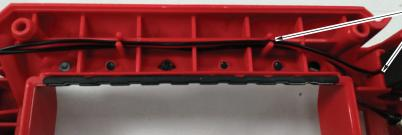
Place the white NTC wires into wire traps as shown.
