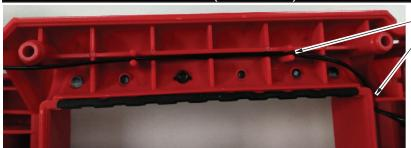
Place the black NTC wires into wire traps as shown.
