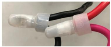
Crimp motor black wire and PCB black wire together using close end connector. Crimp motor red wire and PCB red wire together using close end connector.
