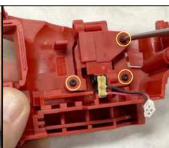
Remove the three M3 T-8 torx screws to separate the switch assembly from the handle support.
