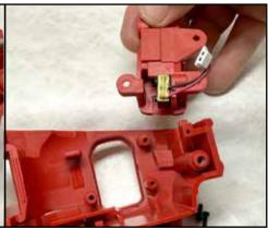
Replace with a new console switch service assembly (23-66-0219). Reassemble by reconnecting wires and following directions in reverse order.
