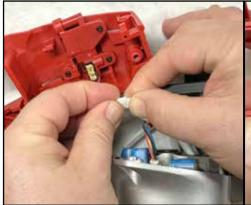
Grasp the switch connector with both thumbs and forefingers and pull apart to separate the handle support/switch assembly from the control board.
