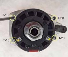
Remove the two M4 T-15 and two M4 T-20 torx screws from underneath the handle to separate the Handle/Electronics from the Motor Housing.
