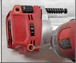
Remove the two M4 T-15 torx screws from the side of the handle cover to separate the handle cover and handle support.
