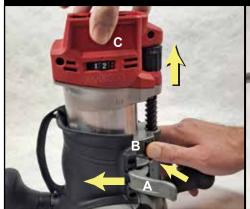
Push the Cam locking lever (A) to the left to unlock the Motor Housing from the Handle Assembly. Push in Spindle Lock Button (B) while pulling up Motor Housing (C) until completely separated from base.
