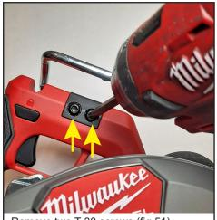
Remove two T-30 screws (fig.51) from rafter hook assembly.
