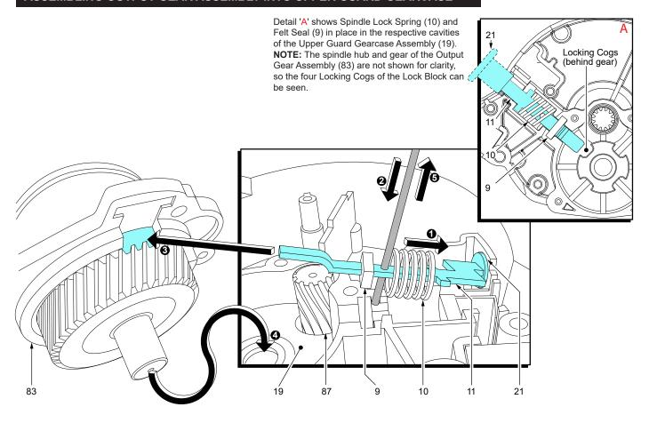
To prevent damage to the Felt Seal (9) it is recommended to temporarily remove the felt seal until steps 1 and 2 are completed.
