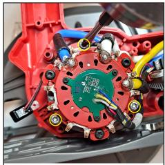
Remove three T-20 screws (fig.47) from stator.
