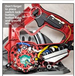
Follow directions in reverse order to put assembly/tool back together. Be sure there are no interferences and wires are properly placed within traps/channels.
