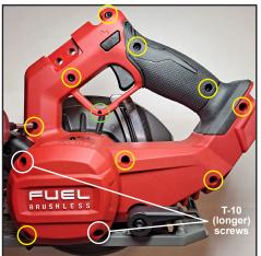
Remove from left housing/handle nine T-15 screws (fig.63) circled in yellow, two T-10 screws (fig.67) circled in white and one T-8 screw (fig.78) circled in green.
