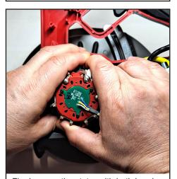
Firmly grasp the stator with both hands and forcibly pull the stator from the magnetic force of the rotor assembly.
