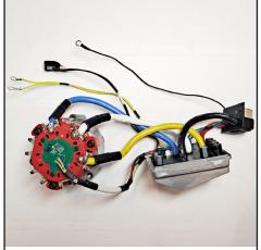
Remove old PCBA & Stator assembly and replace with new PCBA & Stator service assembly 14-46-9964 (fig.85).
