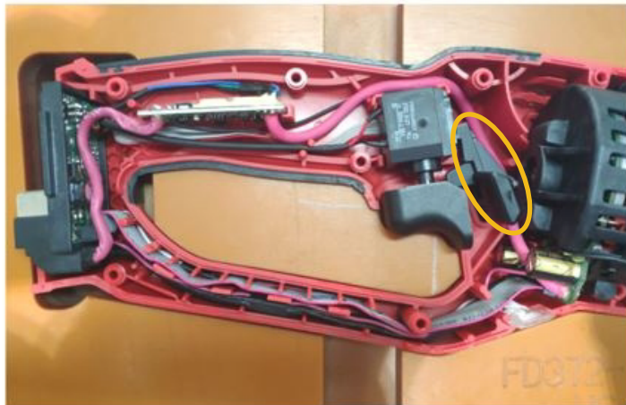
Step 5. Place the Forward/Reverse Shuttle in handle as picture shows above.
