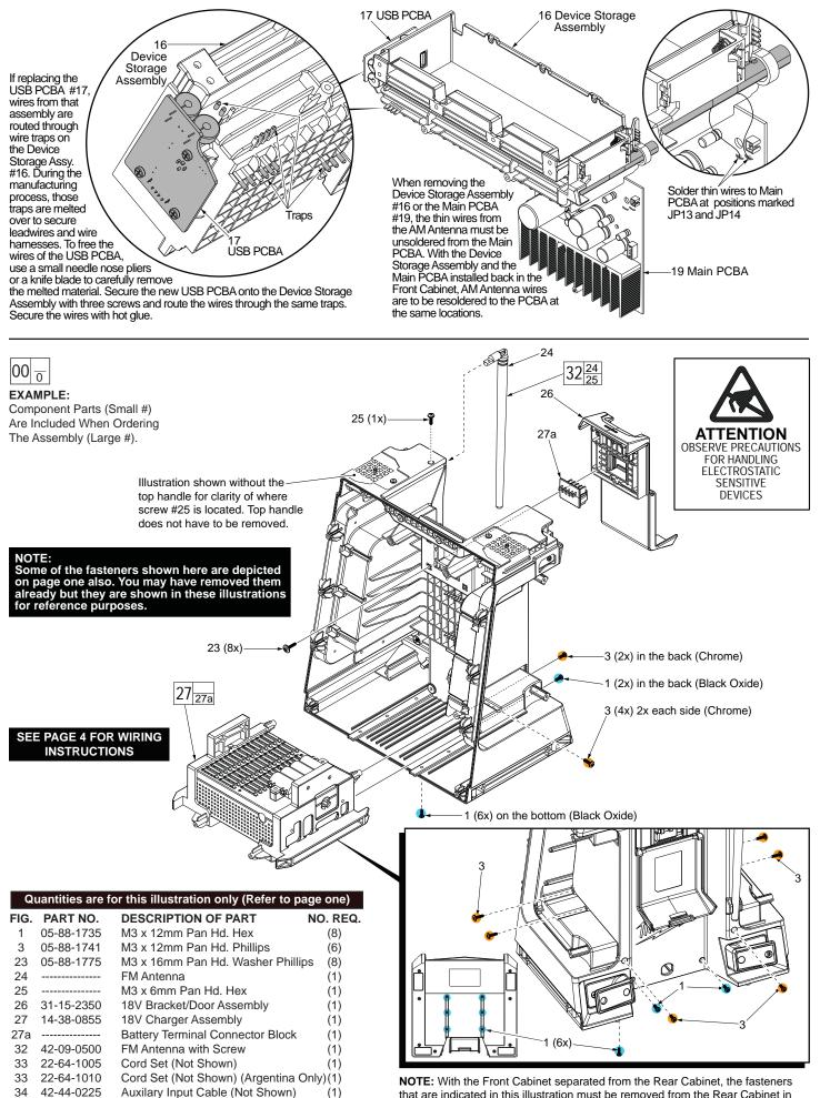
that are indicated in this illustration must be removed from the Rear Cabinet in order to take out the Charger Assembly #27.
