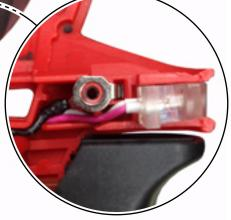
LED wires and HV ground wire are routed through channels and traps behind gear case assembly and forward/reverse shuttle.
