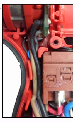
Route wires as shown being very careful to tuck all wires down into traps and behind the on-off switch.
