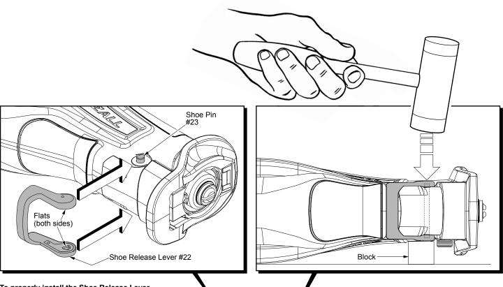
To properly install the Shoe Release Lever #22 onto the Shoe Pin #23 do the following:
