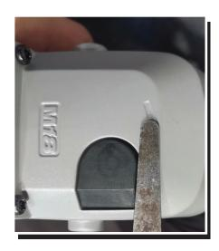
**NOTE** - The surface of the Lock Button **CANNOT** by higher than the surface of the gearcase excessed 1mm.
