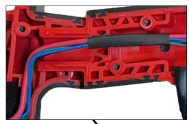
Carefully place/route ribbon cable in traps as shown.
