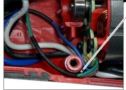
Be careful and do not tighten or strain the wires in this area.
