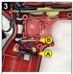
Route wires and place battery terminal (A) and hall board (B) into slots as shown, being sure that they are firmly and squarely seated in the cavities.
