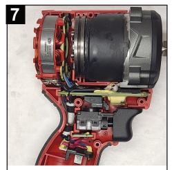
Check that all elements of electronics assembly are seated properly and that all wires are pressed completely down in wire traps and channels.
