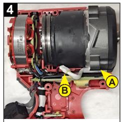
Place gearcase assembly into proper location (A). Attach white wire connectors together (B).
