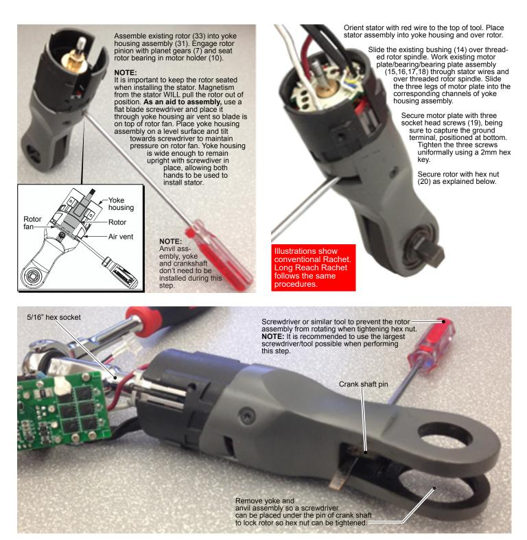
To properly tighten hex nut (20) to rotor (33), it is important to lock rotor and keep it from spinning. The recommended approach is illustrated above.
