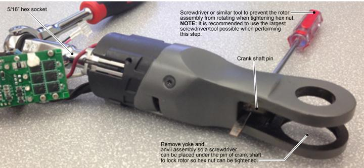
To properly tighten hex nut (20) to rotor (33), it is important to lock rotor and keep it from spinning. The recommended approach is illustrated above.
