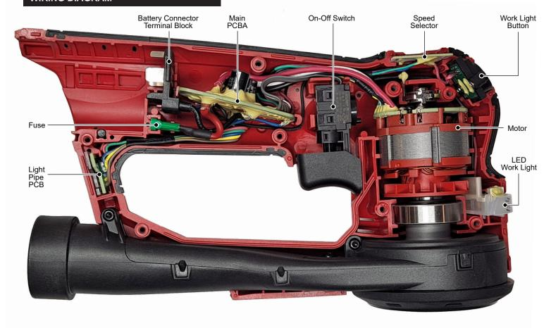
As an aid to reassembly, take notice of wire routing and position in wire guides and traps while dismantling tool.
