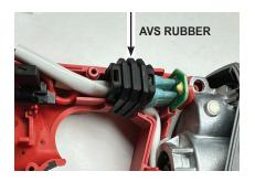
INSTALL THE AVS RUBBER TO THE HANDLE 4X RIBS.
