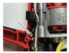
MAKE SURE ALL WIRES ARE IN THE TRAPS AND <u>NOT</u> ABOVE THE SCREW RIB OF HOUSING.
