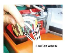
INSTALL THE STATOR WIRES AS SHOWN ABOVE.
