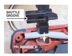
MAKE SURE THE TRIGGER PIN WILL BE IN THE GROOVE OF THE SHUTTLE WHEN ASSEMBLING PARTS INTO HOUSING.
