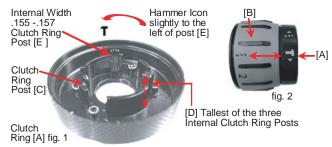
Rear view of (outside) Clutch Ring [A] to illustrate internal Clutch Ring Post widths and positions.
