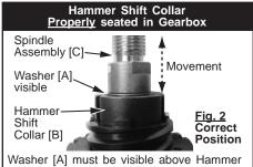
Collar [B] on Spindle Assembly [C]
