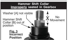
If Washer [A] is not visible, turn collar left or right by hand until it drops into position shown on [fig. 2]. Only one position will allow Hammer Shift Collar to drop down.
