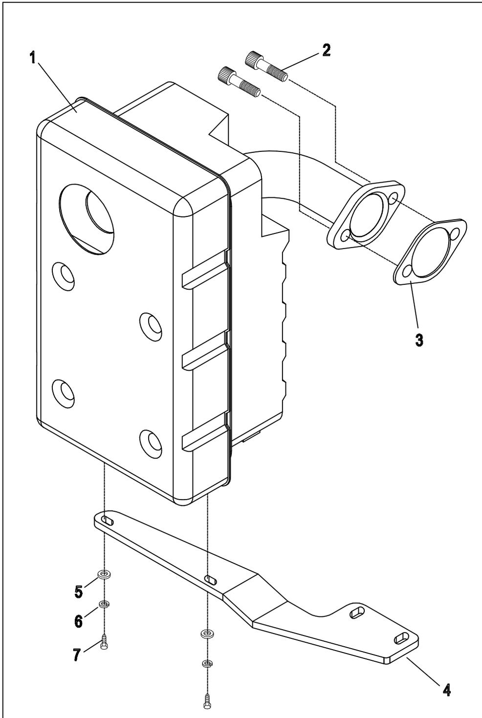
**EXPLODED VIEW: MUFFLER, 410 SIDE OUT
