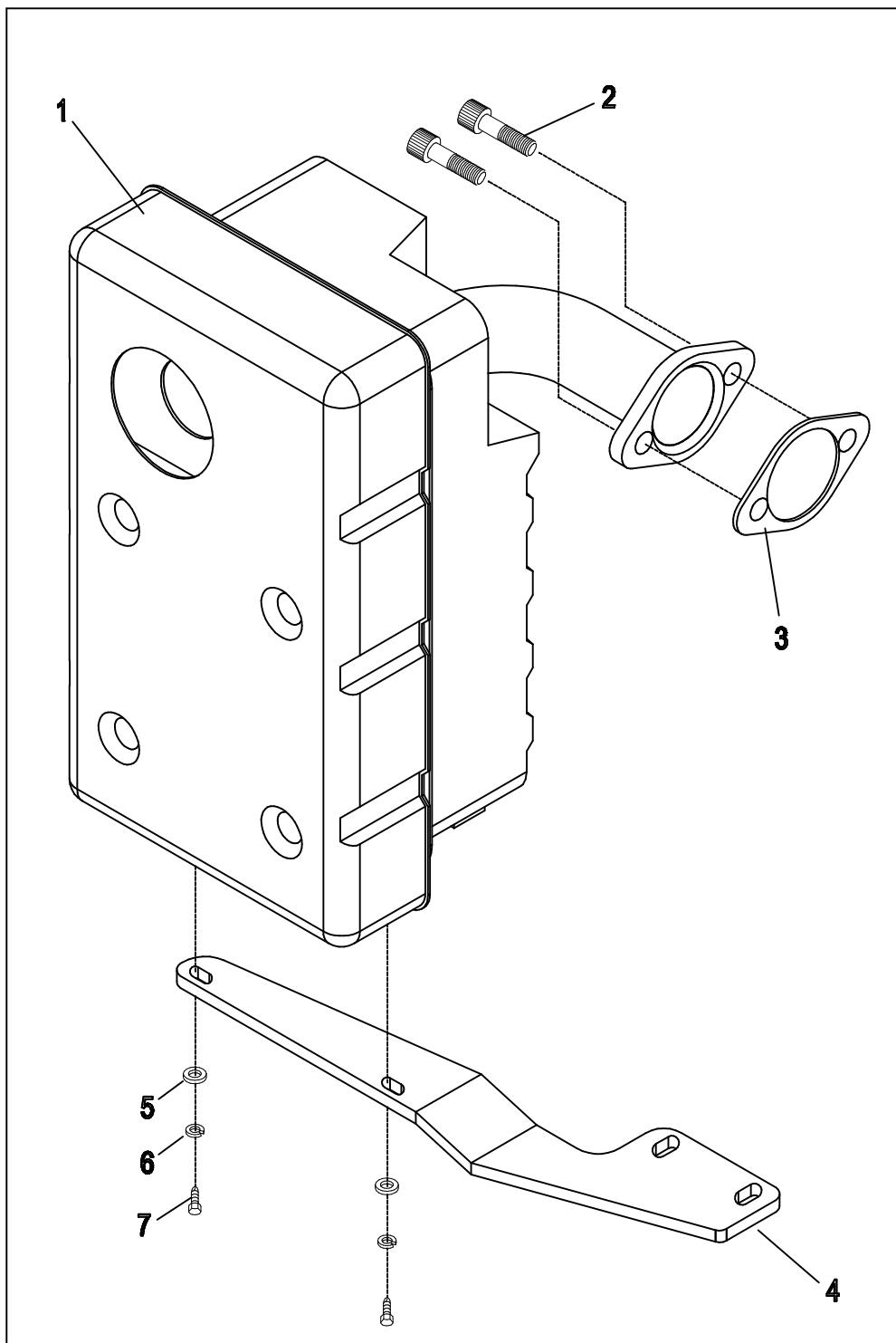
**EXPLODED VIEW: MUFFLER, 410 SIDE OUT****DRAWING #: 0E5081 REV. B****GROUP****APPLICABLE TO:**
